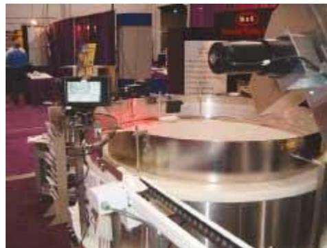
*M&S Automated Feeding Systems is a manufacturer of automated parts feeding equipment. In its latest centrifugal bowl feeder, engineers have incorporated a low-cost image sensor to check a part's orientation before it exits the feeder bowl.*
